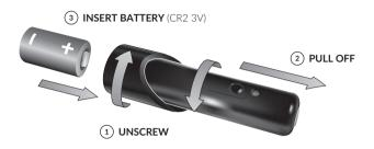
To change the battery, the protective cap and battery cap must be removed and refitted after inserting the battery (see illustration).
